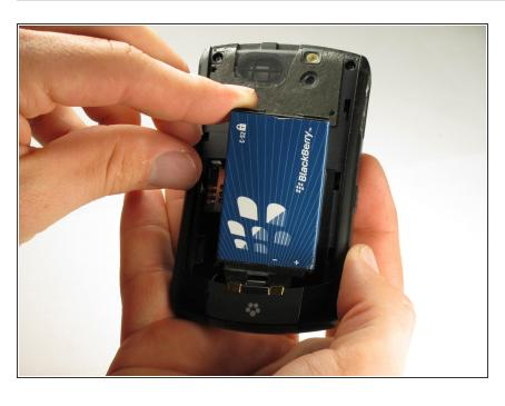
Pull up on the top edge of the battery to remove it.
